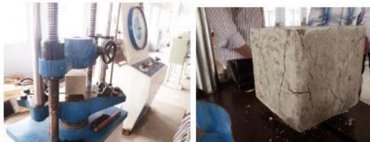
Fig :During Testing And Crack Formation On Specimen
