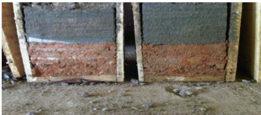
Fig 3: Proper Separation of sub-grade from the sub-base
