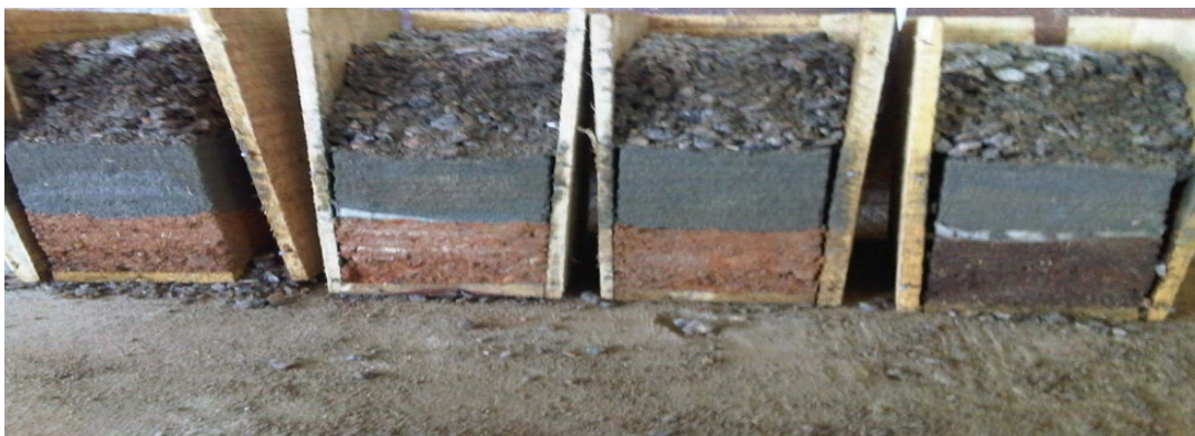
Fig 2: Side view of the pavement models, the 1st on the left without geotextile and the rest with geotextile incorporated
