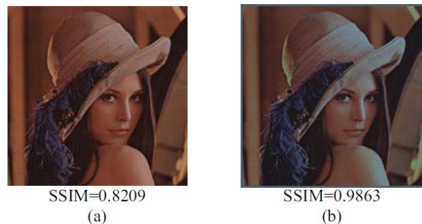
Figure 10: image quality comparison of 'Lena' for different OLED driver designs. (a) Conventional driver (b) DVS friendly driver.
