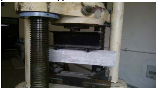
Figure 3.3. Testing of prisms for Flexural strength
