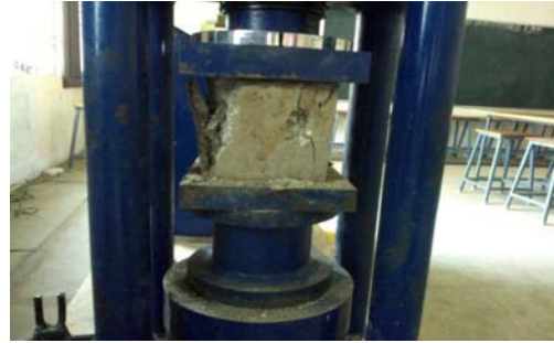
Figure 3.1. Testing of cubes for compressive strength
