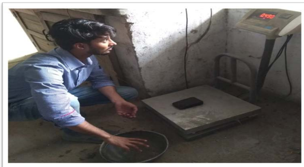
Figure 5: Weight of brick after immersion in water
