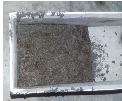
Figure 2: Final mould of brick composite paver
