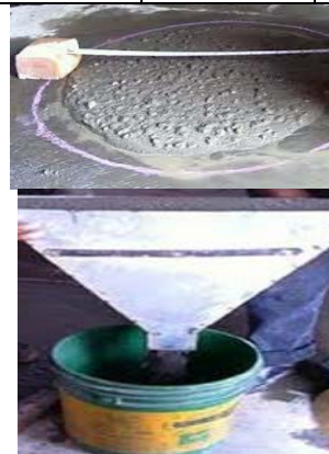
Fig. 5.1 Slump and V-funnel test
