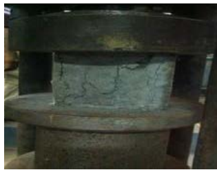
Fig.5.2 Cube under Compression Test
