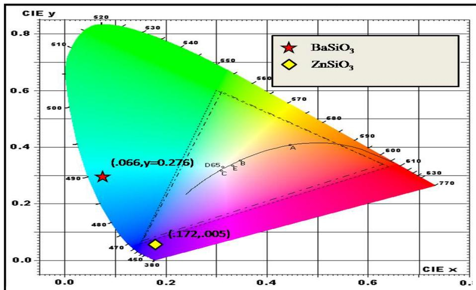
Figure 2 CIE chromaticity diagram of europium doped  $\text{BaSiO}_3$  and  $\text{ZnSiO}_3$  phosphors showing the highest emission intensity at (  $\text{Eu}^{2+}$  = 2 ) mol %.
