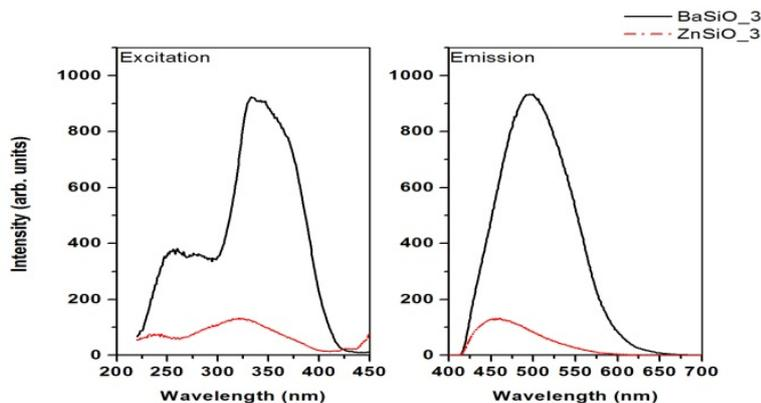
Figure 1 Left side: Excitation spectra for  $\text{BaSiO}_3:\text{Eu}$  (Black) and  $\text{ZnSiO}_3:\text{Eu}$  (Red) sample. Right side: Emission spectra for  $\text{BaSiO}_3:\text{Eu}$  (Black) taken at 354 nm excitation and  $\text{ZnSiO}_3:\text{Eu}$  (Red) sample taken at 325 nm excitation.
