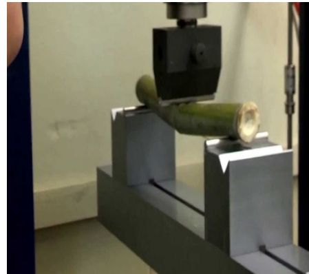
Figure 4. Bending Strength Testing
