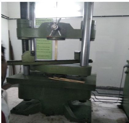
Figure 2. Tensile Strength Testing
