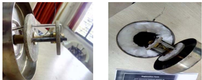
Figure 6 -a) Sample Holder, b) Complete view of Sample Holder with furnace.
