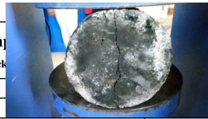
Figure 4.2 Split tensile test
