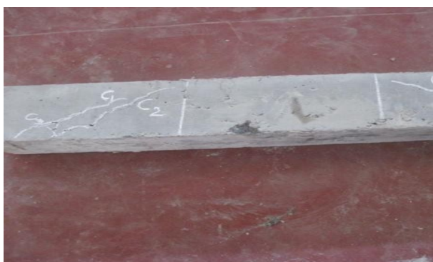
Fig 5 Cracks on control specimen
