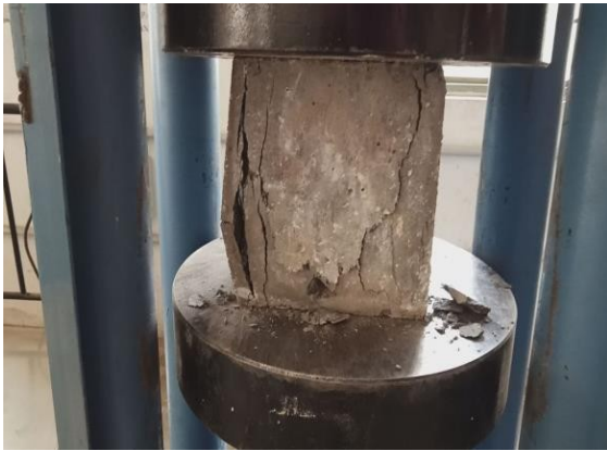
Fig 3 compression test on beams
