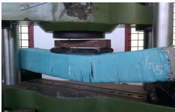
Fig 6 Failure of Retrofitted beam
