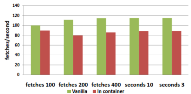
Fig 3: Performance evaluation using http load. The overhead is between 10.3% to 26.2%
