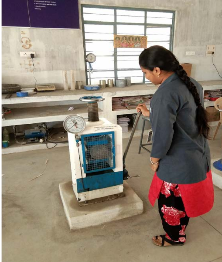
Fig No 5.14 :Testing of Cylindrical specimen
