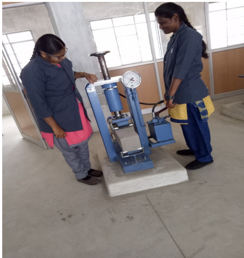
Fig No 5.14 : Testing of prism specimen
