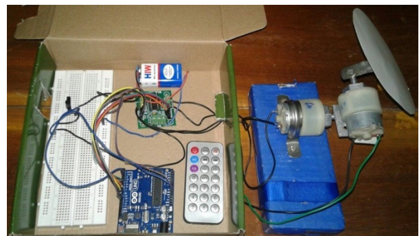
Fig. 4. Implemented Model of Dish Position Controller Using TV Remote
