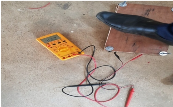
Figure 5.3(b) Piezoelectric Transducer output
