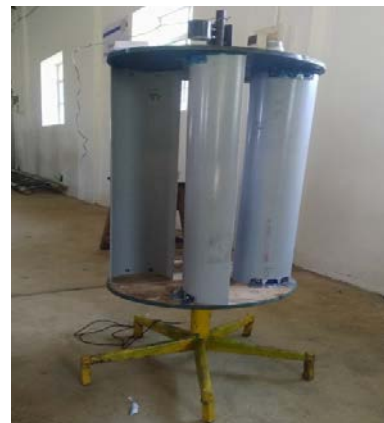
Figure 5.4(a) Vertical axis wind turbine
