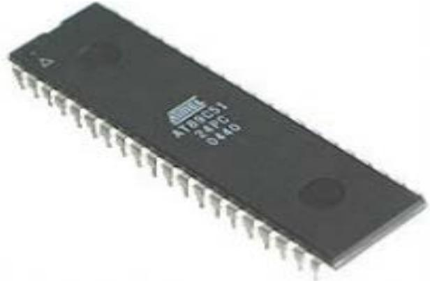
Figure.2 Atmel 89C51
