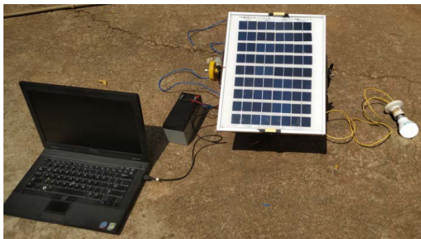
Figure 4.1: Figure shows the single axis solar tracker
