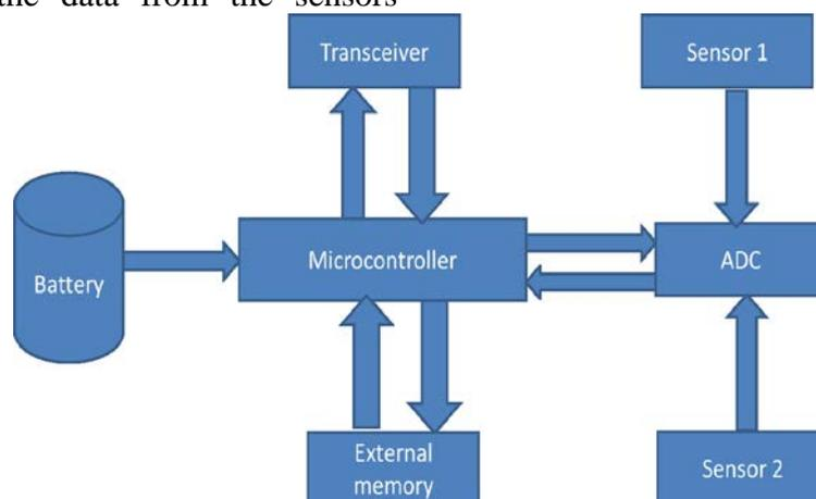
**Figure 1 Block diagram of a node in agricultural WSN**
