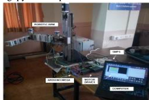
Fig.10 Experimental setup of SCARA Robot.
