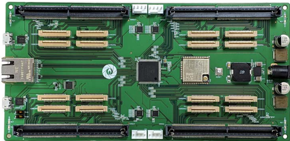
Figure 3: 16 1080p 30fps video streams in a single board modular design approach allows you to take advantage of standardized electrical connections between modules when designing your board. [9-10]
