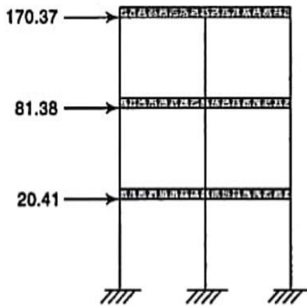
Figure 3.2: Problem Validation Lateral Forces
