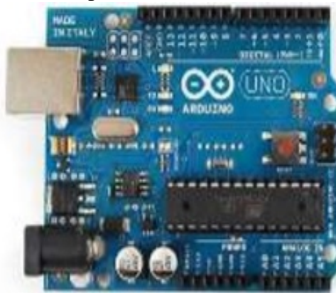
Fig. 2: Arduino Uno Microcontroller Development Board
