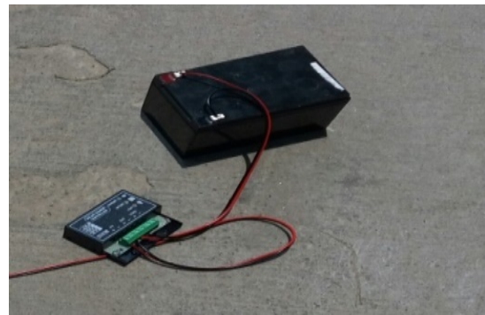
Fig.9 battery and charge controller
