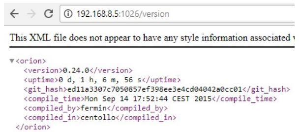
Figure 6: Confirmation of the execution of the Orion Context Broker service. http://192.168.8.5:1026/version (The corresponding port 1026 is the Broker's listening port)
