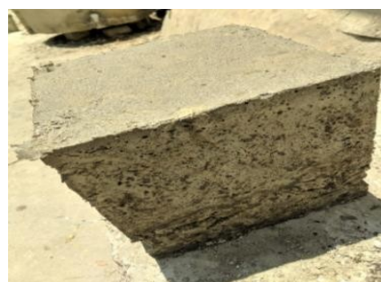
Fig4: Demoulded cube Specimen
