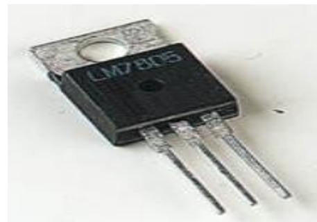
Figure 1.5 Three terminal voltage regulator
