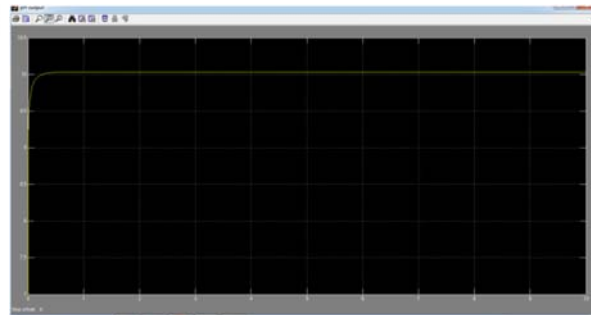
Fig. 15. Response obtained from the system with Fuzzy controller tuned for an operating point at pH=10
