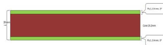
Fig.7 Material Properties of composite sandwich panel –Mono core
