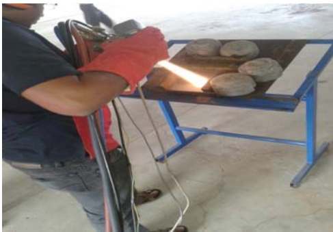
Fig.6 HVOF Spraying Process
