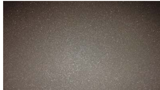
Fig.4 Grit blasted sample surface
