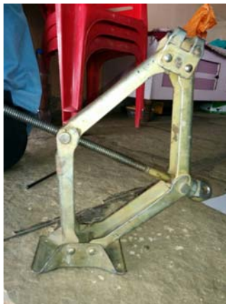
Fig. Toppled Scissor Jack due to Arm teeth Failure
