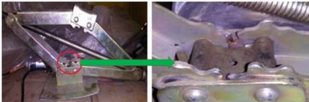
Fig. Failure of Screw and Arm Teeth
