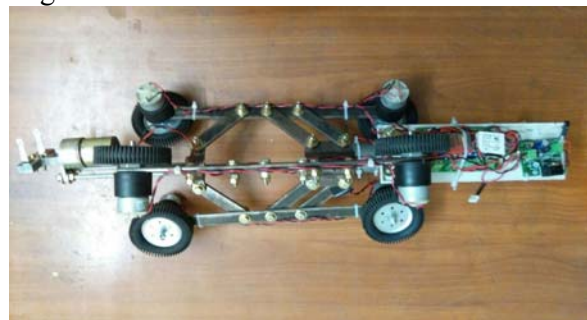
Fig.17 – Fully assembled pipe inspection robot Working: The complete assembly of the robot leads to the next phase of the project – Working.
