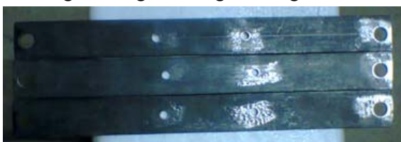
Fig. 9 – Holes drilled on link 1
