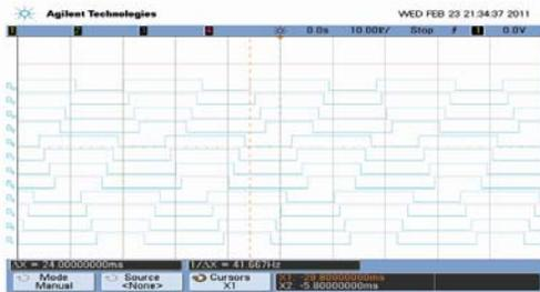
Fig. 3. Gating signal generation (switching pattern) for 3-level inverter
