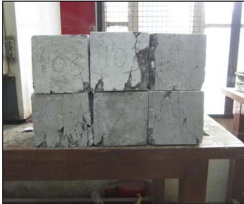
**Fig.3:Typical Mode of Failure for Cubical Specimens.**
